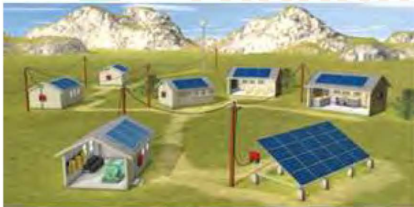
Fig. 3: Concept of a solar mini-grid in a rural set up
