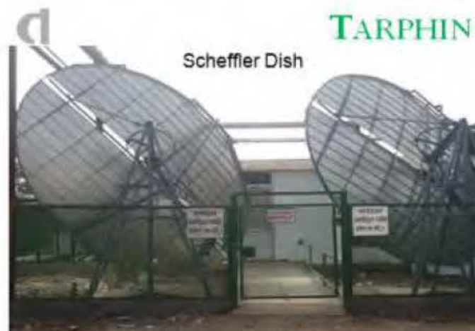
Fig. 6 : Schaeffler concentrators developed by TARPHER
